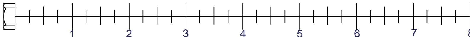
(A4)HEX BOLT 1/2"x3 1/4"L PARTIAL THREAD QTY.14
